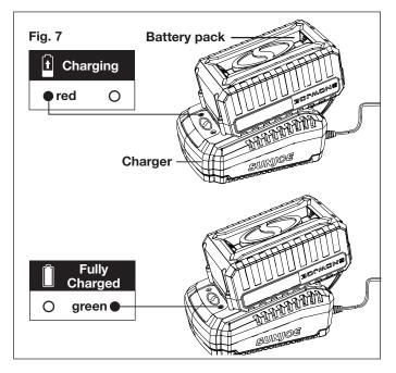
**4.** When the charger light turns green, the battery is fully charged (Fig. 7).
