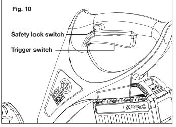
**3.** To stop the cordless snow shovel, release the trigger switch.
